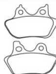
MX400 A 97.5 x 64 x 8mm B 97.5 x 64 x 8mm HH = 7.5mm thickness
