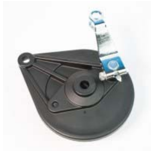
PORTA BALATA DELANTERO COMPLETO P/ XT-110RT II '17-'19, P/ XT-110RT '20, P/ AT-110RT '13-'14, P/ XT-125RT '20
