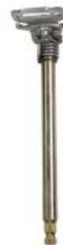
FLECHA DE VELOCIDADES P/ DM-200 '14-'21, P/ DM-200 SPORT '19-'20, P/ DM-150 SPORT '19-'20, P/ DM-125 '17-'20
